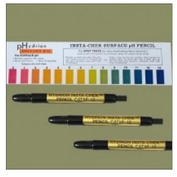
To measure the surface pH just wet the surface with distilled water. Stroke the surface with pencil. Wait approximately 15 seconds and compare the resulting color change with the color chart.
